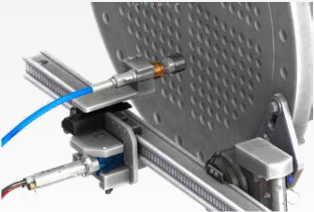
SHOTGUN MOUNT For surface prep and tube sheet cleaning.
